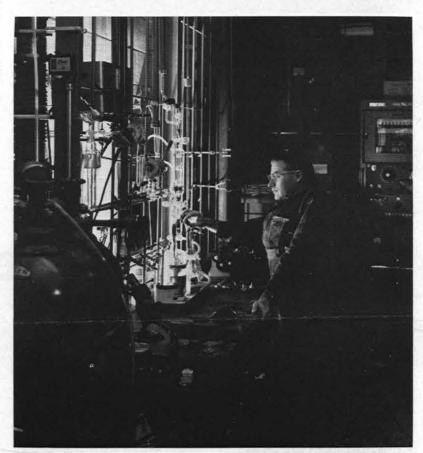
HIGH VACUUM system, recently completed at the Livermore Laboratory chemistry lab, is operated by Charles Arthur (8815-2). The system was designed to determine the hydrogen, nitrogen, and carbon contents of organic materials present in test samples.
